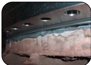
Gasket chocking using 101 Power Metal Repair Paste
