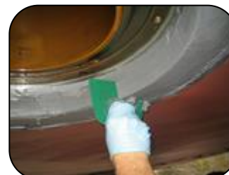
Metal surfaces resurfaced using 101 Power Metal Repair Paste
