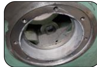
Metal surfaces rebuilt and machined using 101 Power Metal Repair Paste
