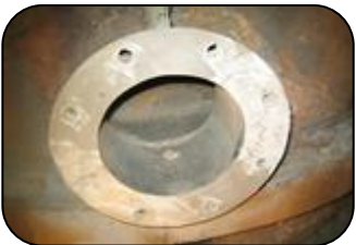
Flange face reforming using 101 Power Metal Repair Paste
