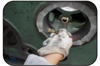
Metal surfaces rebuilt and machined using 101 Power Metal Repair Paste
