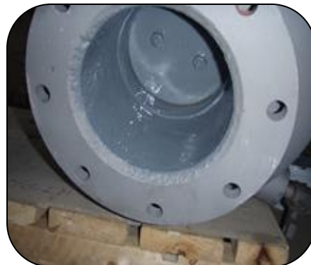
De-sulphurisation unit operating at 167°F (75°C) rebuilt using PES 201 Ceramic Repair Paste and resurfaced using PES 205 Ceramic HT Fluid
