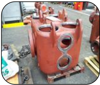
Sea water filter operating at 203°F (95°C) coated with PES 205 Ceramic HT Fluid
