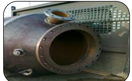
De-sulphurisation unit operating at 167°F (75°C) rebuilt using PES 201 Ceramic Repair Paste and resurfaced using PES 205 Ceramic HT Fluid
