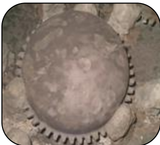
Ammonia Liquor process vessel operating at 212°F (100°C) resurfaced with PES 205 Ceramic HT Fluid
