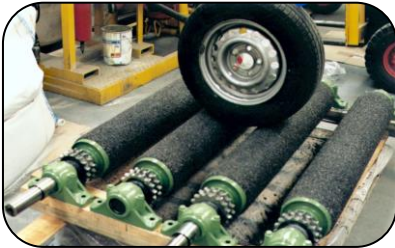
Resurfacing of brake test rollers using PES 102 Power Metal Repair Fluid
