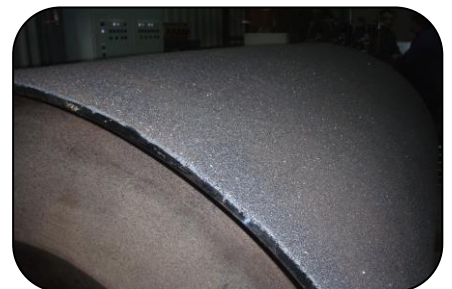
Damaged tank seams filled and rebuilt using PES 102 Power Metal Repair Fluid
