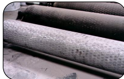
Belt rollers resurfaced using PES 102 Power Metal Repair Fluid and Aluminium Oxide
