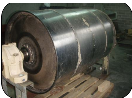
Resurfacing of brake test rollers using PES 102 Power Metal Repair Fluid
