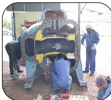
Split case pump rebuilt and protected using PES 201 Ceramic Repair Paste and PES 202 Ceramic Repair Fluid
