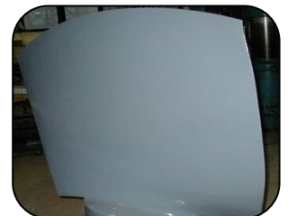
Turbine blades protected using PES 202 Ceramic Repair Fluid
