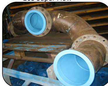
Process pipework abrasive blast cleaned and coated with PES 203 Super Flow
