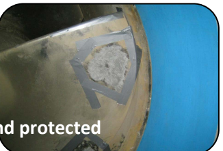
Rudders resurfaced and protected
