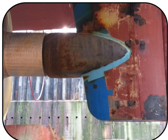
Rudders resurfaced and protected
